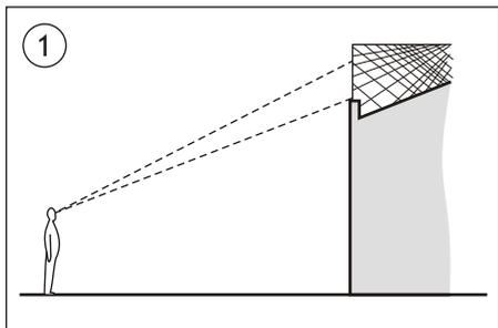
In this example (1) the netting has been located from the top of the parapet to a height that can encompass the whole pitch of the roof. This means that the netting will be clearly visible from the street.
