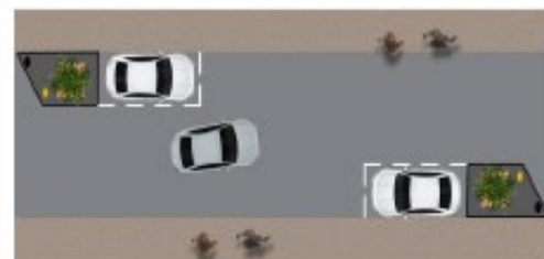
Schematic diagram showing chicane parking with build-outs
