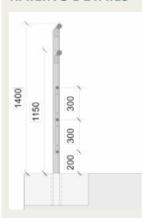
1400mm railing with posts at 2200mm centres. Vertical reinforcement made from 15mm steel bar, welded to tubes. Posts to be fixed into capping beam by drilling circular hole and filled with epoxy grout. Fixing design to be demountable.
