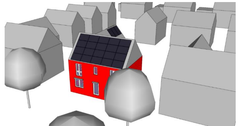
A 3D model of the house and surrounding features was created in DesignPH 2.1.15 and used to calculate solar gains and shading for PHPP.
