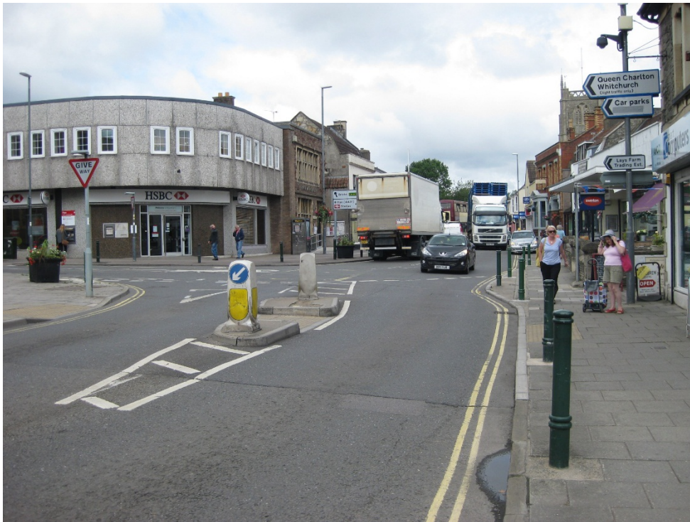
Behaviours at the entrance to the High Street vary, with some vehicles barely slowing down, and a limited number stopping to allow pedestrians to cross. Bollards, signs and street furniture result in a visually cluttered view. Road narrowing and deflection would slow vehicles down and allow pedestrians to cross more readily.
