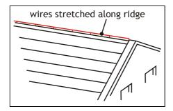
Wires need to be sited sensitively. Skylines that are visible from prominent public places should be avoided (see Netting). Bright colours may improve performance but should not be used. This sort of system needs to be properly installed and maintained if it is to be successful. If done incorrectly, gulls can still enter the excluded area
